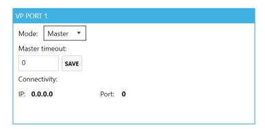
If the VP Port is set to work in "Master" mode, the VP Processor will use that port as a regular output, so data will be sent to the first VP fixture in the cabled string.
