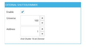
3 more DMX channels can be added to the VP fixture selected: one "master" Shutter or Strobe channel with 8 Bit resolution, and a General Dimmer with coarse and fine DMX channels (16 Bit).
